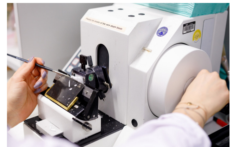
Sectioning a paraffin block using a microtome
