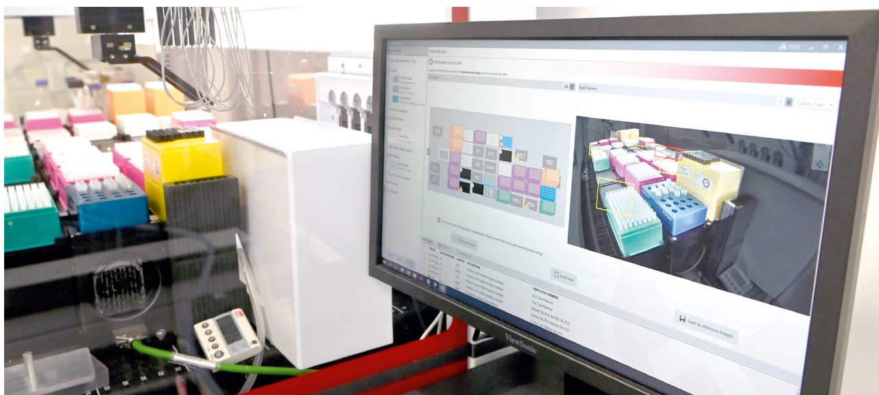
Automation using the 384-head liquid handling robot Biomek i7 opened the door to the miniaturization of sample preparation protocols.
